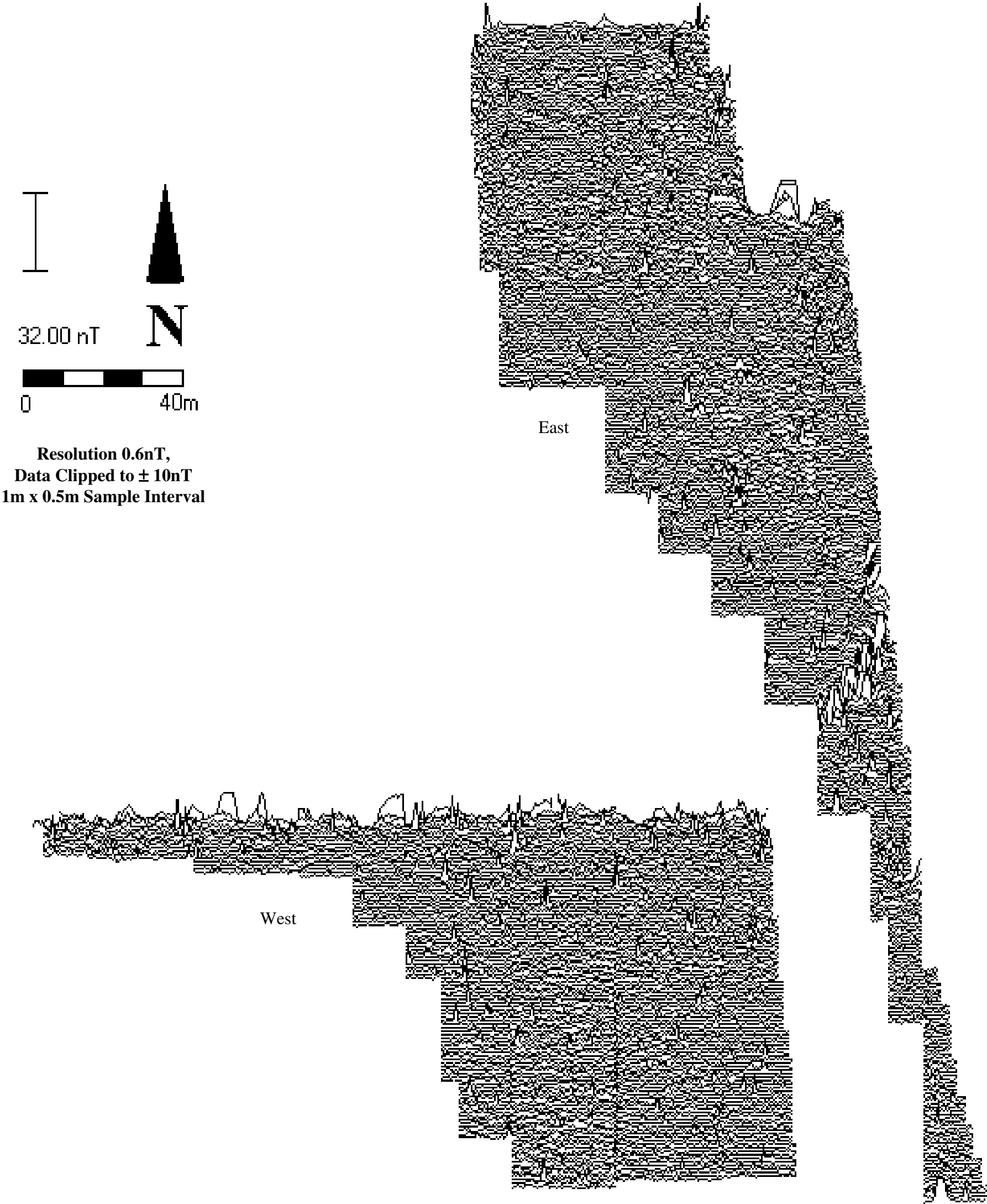
Figure 02: Pre-processed Fluxgate Gradiometer XY Traceplot of Site 4
