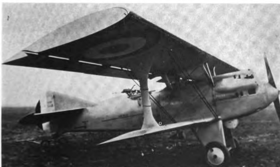
FRENCH AIRPLANE EQUIPPED WITH SLOTTED WINGS GIVING IT A SLOW SPEED. THE AIRPLANE HAS A MAXIMUM SPEED OF 132 MILES PER HOUR AND A MINIMUM SPEED OF 43 MILES PER HOUR
