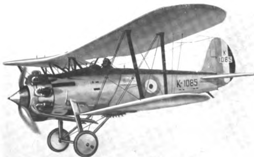
BRITISH SINGLE-SEATER PURSUIT PLANE CALLED THE "BRISTOL" WHICH HAS A SPEED OF ABOUT 180 MILES PER HOUR AND A CEILING OF 31,000 FEET
