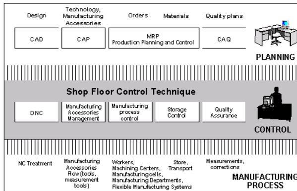
Fig. 23 Tasks of Shop Floor Control Technique (SFC) [1]
