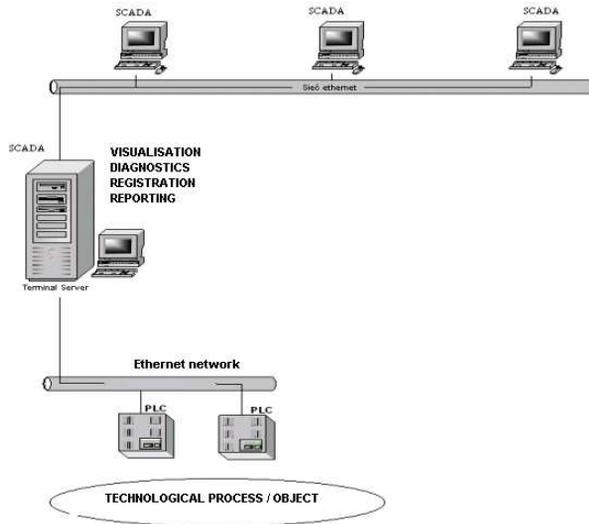
Fig. 37 SCADA System – a system of control, managing and data archiving [66]
