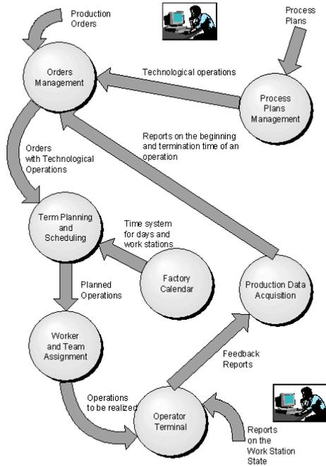
Fig. 43 Scheme of SFC system functioning [4]
