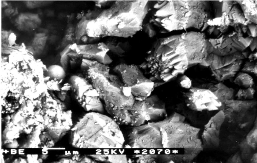
Fig.2. Example of limestone pore space morphology under the scanning electron microscopy (SEM). In central and upper part there are visible secondary calcite crystals; on the left – gypsum crystals and dust spherules.
