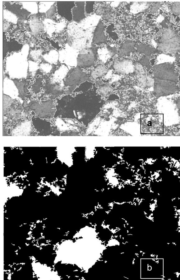
Fig.1. Microphotograph of sandstone sample. Image analysis helps detecting pores in the sample: a – image transformed into grey colours with contoured pore areas, b – binary map of the previous image
