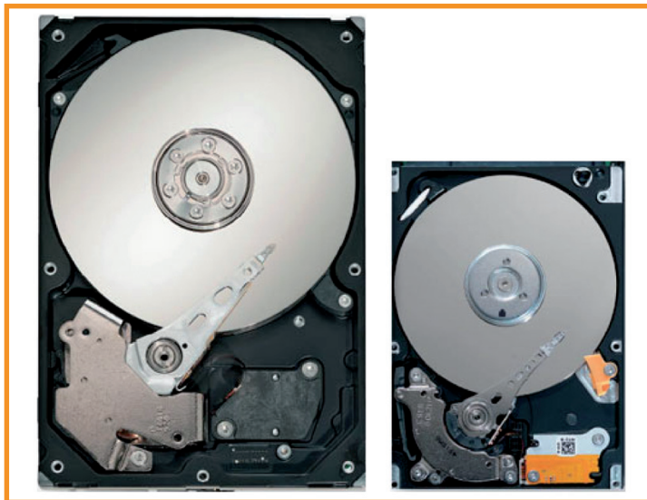
Fig. 9. A 3,5" hard disk drive used in PCs (left) and a 2,5" one used in laptops (right)
