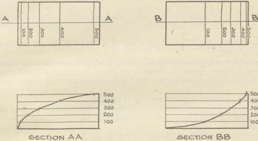
FIG. 9.—CONCAVE AND CONVEX SLOPES
