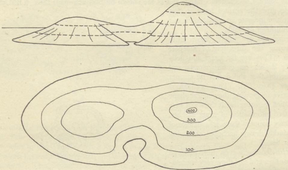
FIG. 7.—DIAGRAM AND CONTOUR SKETCH-MAP OF AN ISLAND
