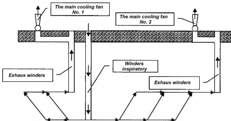
Fig. 1. A model diagram of ventilation network A
