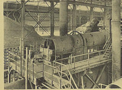
**6** Conditioner and operating platform of 1,000 ton granulating unit showing spray valves, flood light, and instrument panel
