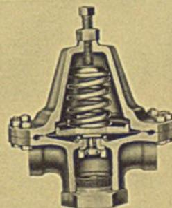
Cash Standard Type 8871 Pressure Reducing Valve; for use with liquids—especially dirty liquids, like Bunker C fuel oil for example. No sliding fits; inner valve bolted to diaphragm for positive movement.
