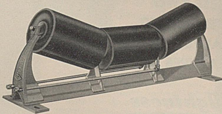
There is a size and type of Continental Idler for every Belt Conveyor application. All idlers, regardless of type, have several improved features common to all. Idler Rolls of all types are easily removed from supporting brackets by simply lifting them out, which can be done with five and six-inch diameters of either cast iron or steel to suit conditions, and of course are equipped with "anti-friction" bearings.
