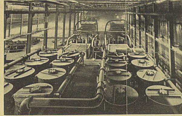
**5** Contact acid production has been added partly to supplant and partly to supplement the chamber capacity
