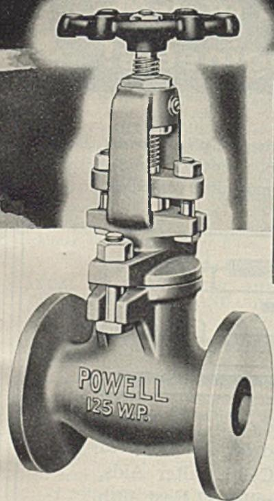
**Fig. 1911**—Flanged End O. S. & Y. Gate Valve with outside screw rising stem, bolted yoke bonnet and nested gasket. Made in sizes  $\frac{1}{4}$ " to 2", inclusive, for 125 pounds W. P. Also available with screwed ends—Fig. 1910—in sizes  $\frac{1}{4}$ " to 2", inclusive.
