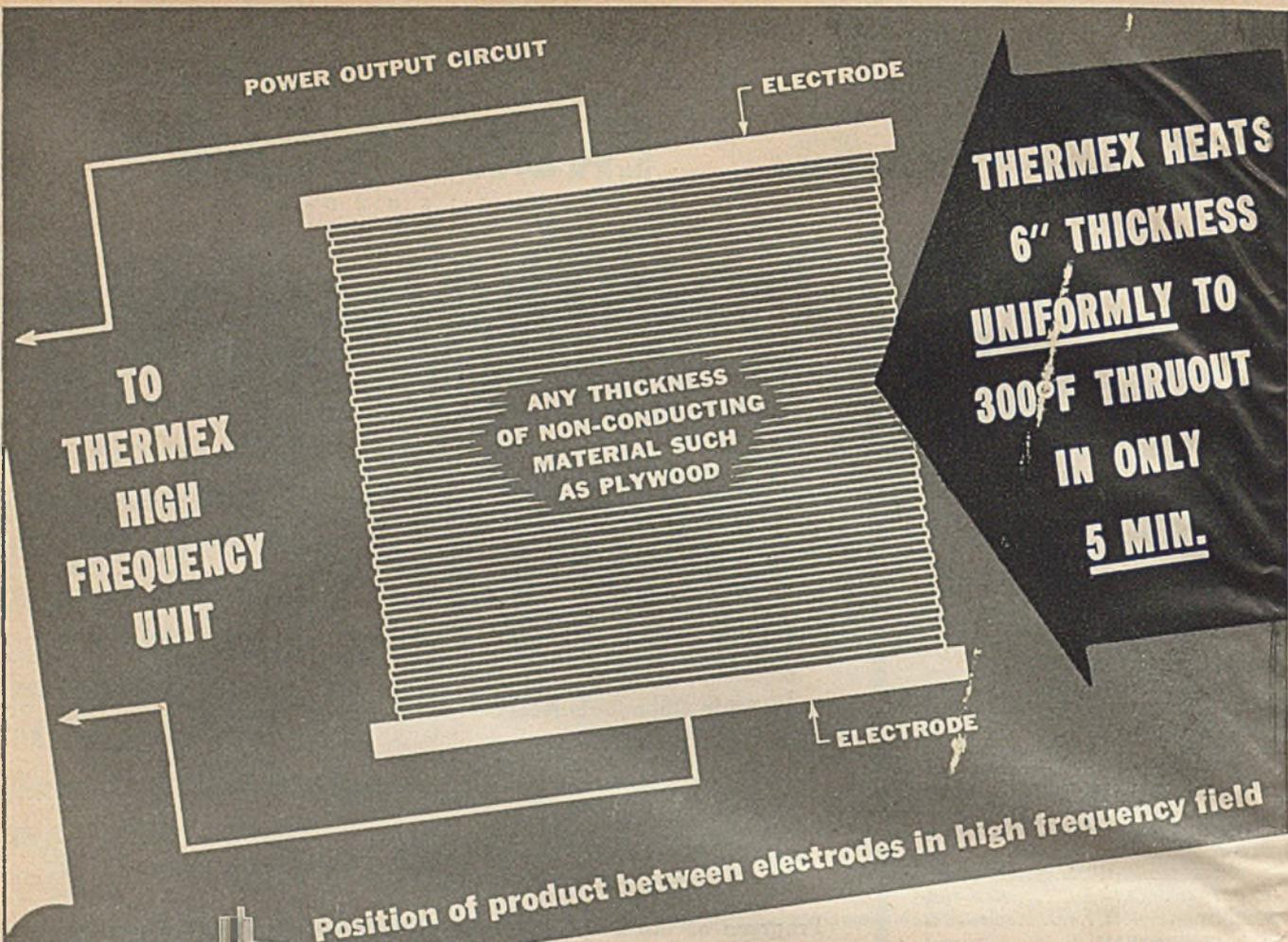
Position of product between electrodes in high frequency field
