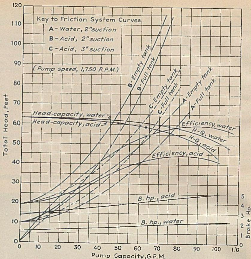
Fig. 3—Head-capacity and friction system curves for water and acid, showing typical capacity decrease and power increase when handling a viscous liquid
