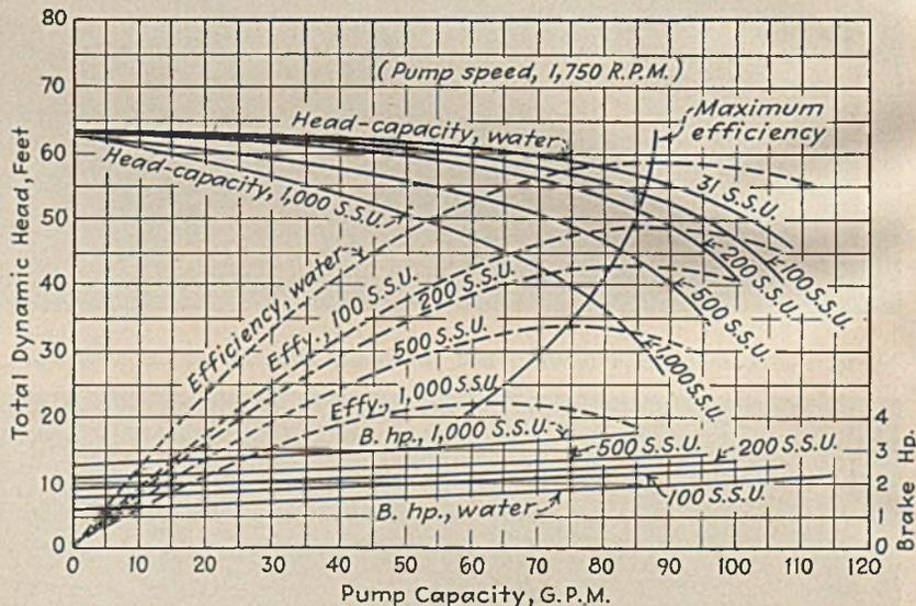
Fig. 4—Variation of performance with viscosity in a typical 2-in. closed-impeller pump of the type used for handling strong sulphuric acid
