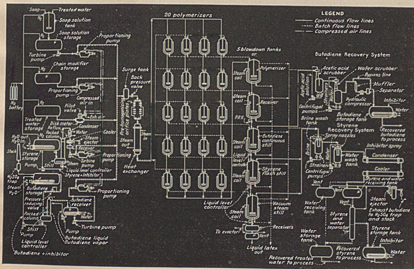
at 50 deg. F. and condensed in the receiver at 35 deg. F. The packed tower effects both a thermal separation of butadiene vapors from the inhibitor vapors, and a mechanical separation of entrained inhibitor. The inhibitor, dissolved in the butadiene reflux, is pumped back to the butadiene tank.
