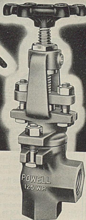
**Fig. 1918**—Screwed End O. S. & Y. Angle Valve with outside screw rising stem, bolted yoke bonnet and nested gasket. Sizes  $\frac{1}{4}$ " to 3", inclusive. Also available with flanged ends (Fig. 1919), and in Globe pattern (Fig. 1912 with screwed ends, Fig. 1913 with flanged ends.)
