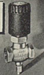
These two-wire, current failure, pilot-operated valves are capable of handling large capacities with a minimum pressure drop. The main valve is held open electrically, eliminating undue pressure loss. Manual opening device incorporated in design. Available for any voltage, AC or DC. Packless design; coils separable. Available 3/8" to 1/2" I.P.S. Ask for Catalog No. 52.
