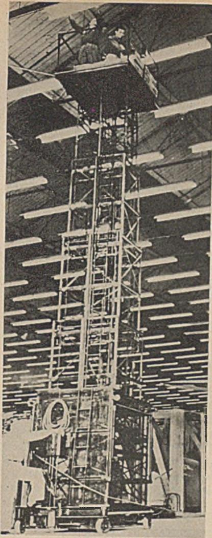
This movable extension tower-platform is a convenient means for servicing the lighting units in a plant
