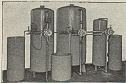
**PHARMACEUTICAL PLANT.** Capacity: 1,700 gallons per hour. Other units have permissible flow of 100 gallons, increasing up to 50,000 gallons output per hour.
