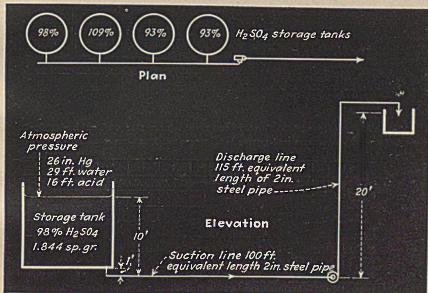
Fig. 2—Friction losses with water and 98 percent sulphuric acid in steel pipe
