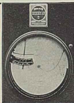
Why worry with factors and "microscopic" low rate readings when all Simplex MS meters use an evenly spaced chart—with even graduations from 0 to maximum.
