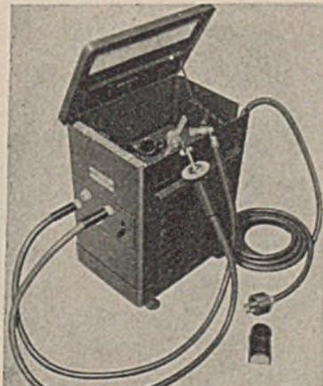
The equipment fuses a rough deposit of electrode metal on to the surface to be metallized, electrodes being applied to the work with a special holder which uses up to six electrodes at one time, depending on the size and nature of the part to be prepared. Small parts, it is stated, can be prepared as easily as large shafts, since there is no excessive heating of the base metal or disturbance of its physical characteristics.
