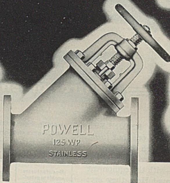
**Fig. 1944**—Flanged End O. S. & Y. "Y" Valve with outside screw rising stem, threaded-through bronze yoke bushing, full, round, bolted flanged yoke bonnet and nested gasket. Made in sizes  $2\frac{1}{2}$ " to 12", inclusive, for 125 pounds W. P. Body can be provided with cleanout pockets on special order.
