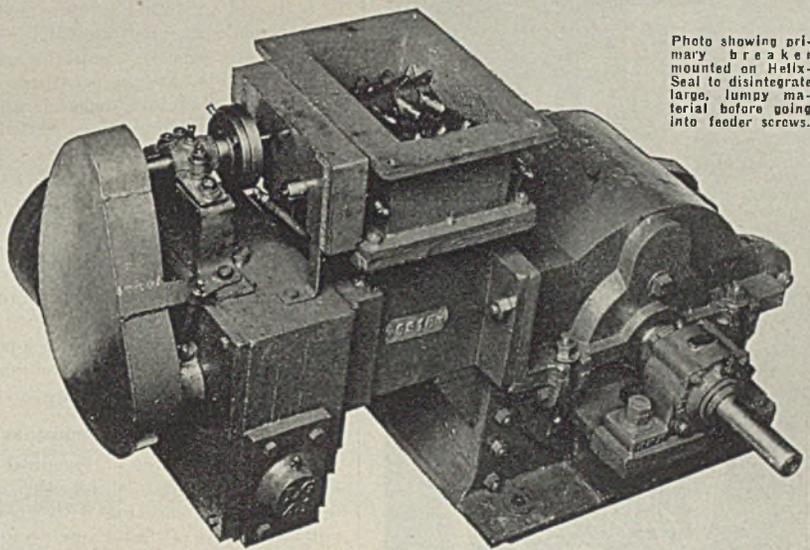
Photo showing primary breaker mounted on Helix-Seal to disintegrate large, lumpy material before going into feeder screws.
