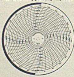
12" circular chart for daily or weekly removal. Electric or mechanical clock drive.
