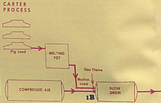
**1B** In the Carter process the lead is atomized to expedite corrosion. By this process white lead can be produced in 12 days
