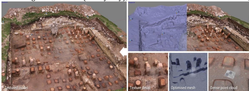
Figure 4: Image processing work-flow to obtain high resolution textured models.
