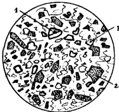
Fig.41 - Refractor cromo-magnezitic: 1-periclaz, 2-spinel, 3-forsterit; N II, ~ 40 x
