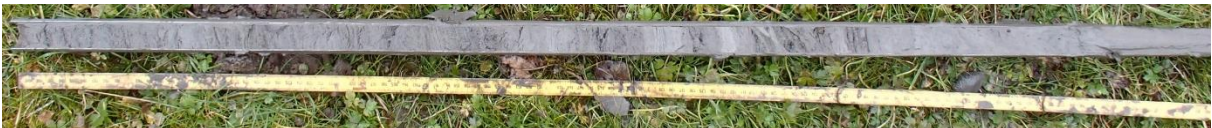
Boring 3: Detail steekguts restgeul opvulling.
