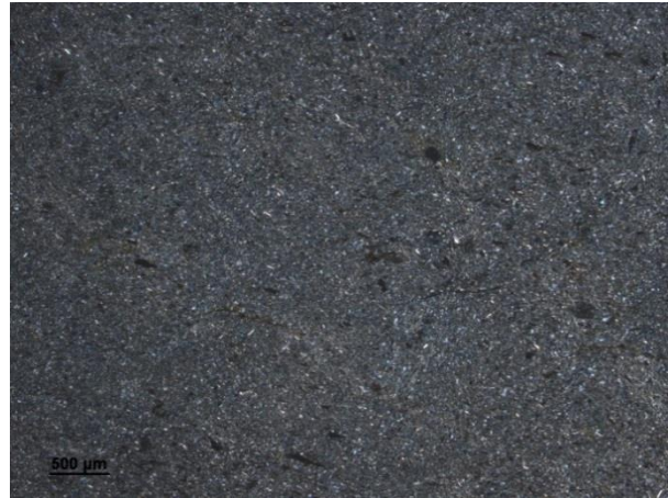
11.4: Dichte homogene matrix (XPL)
