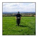
probes reach each designated sample interval. Surveys are usually undertaken at 1 m sample intervals along 1 m traverses (i.e., 400 readings per 20m  $\times$  20m grid. The adaptability of the instrument enables increased sampling intervals, as well as a range of probe configuration to operate at varying depths.
