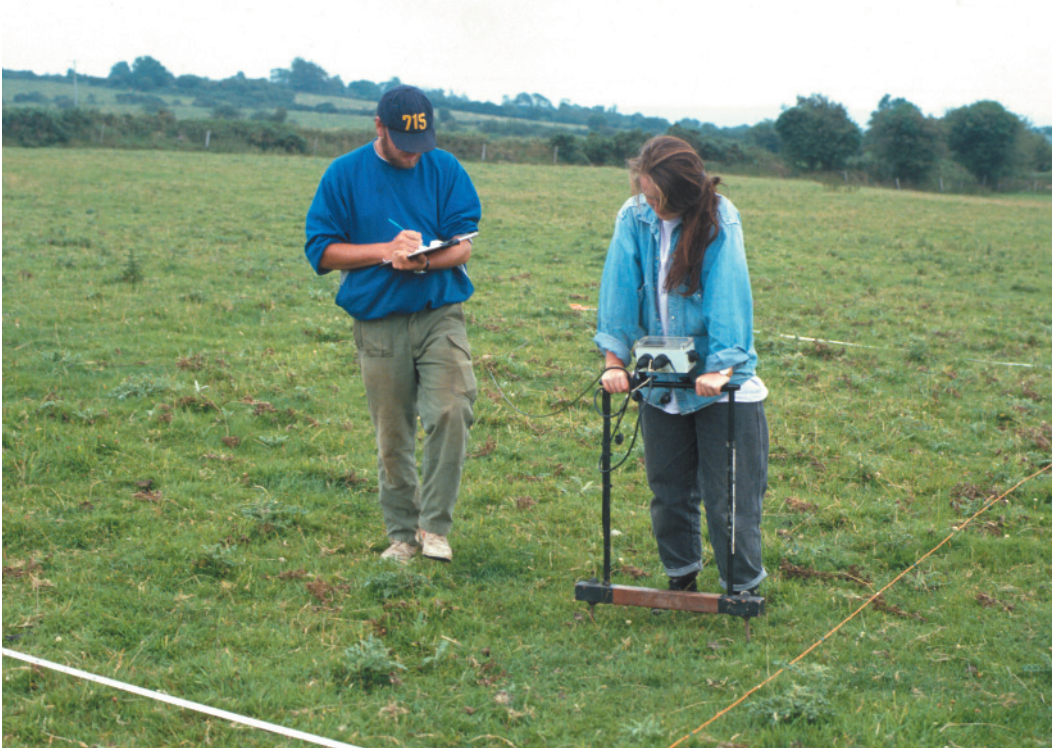
Electrical resistance twin-probe array (Kevin O'Callaghan)
