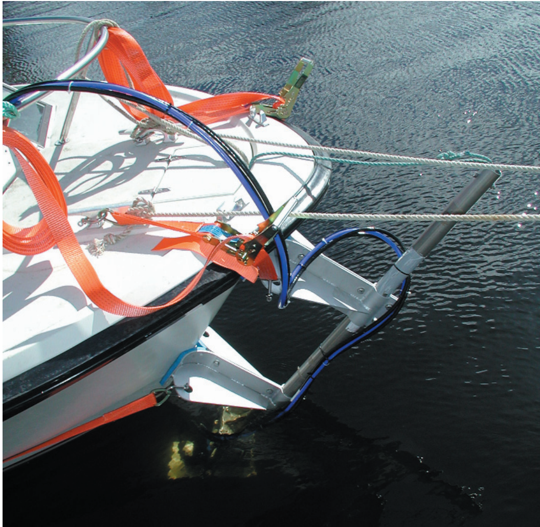
Multibeam echo sounder transducers mounted on the bow of a shallow-draft survey vessel (Shane Rooney)
