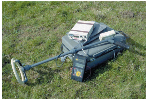
Magnetic susceptibility equipment including measurement console, 20 cm fieldloop and datalogger (Shane Rooney)
