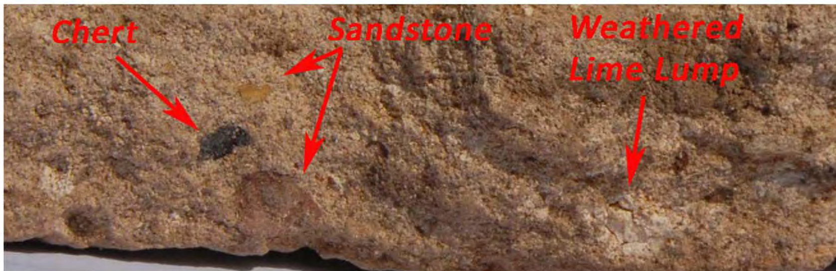
Plate 48: Sample No 7, Area A, Deposit 52 General view of the mortar matrix
