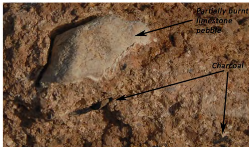
Plate 55: Sample No. 15, showing charcoal and partially-fired limestone grains
