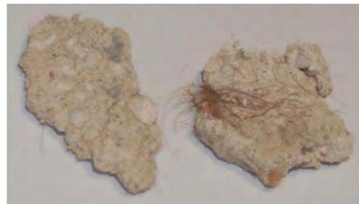
Plate 75: Sample No 129, showing lime lumps and hair
