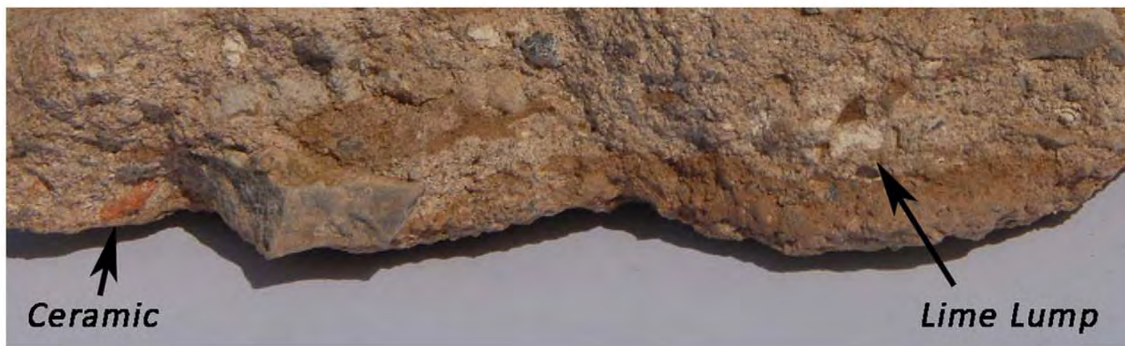
Plate 47: Cermaic (pozzolanic) fragments and lime lumps in Sample No 3, Area A, Deposit 52
