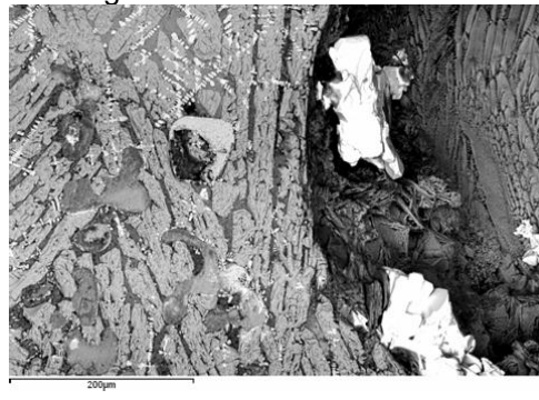
SEM-BS image of a section of 323.9 image 7 showing bright barium sulphate inclusions
