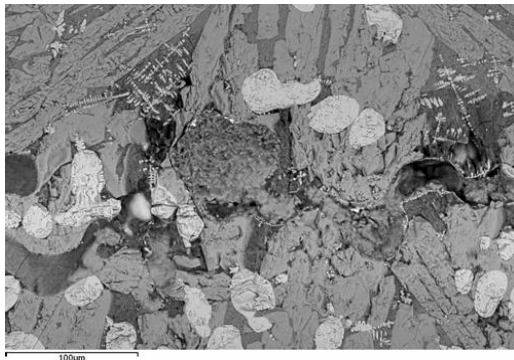
SEM-BS image of a section of 323.9 image 8 showing particle of un-reacted/partially reacted ore in the middle of the fayalite needles, wustite and interstitial glass
