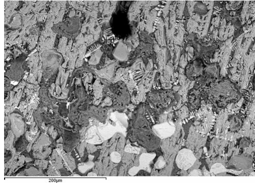
SEM-BS image of a section of 323.9 image 2 close up of image 5; the sample is heavily weathered as can be seen from the rough surface of the mineral grains and the interstitial glass.
