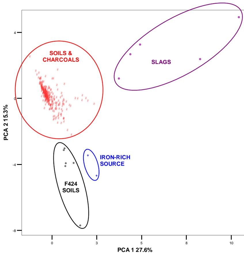
**Figure 7.** Principal components analysis plot for all materials, using all elements determined by XRF.
