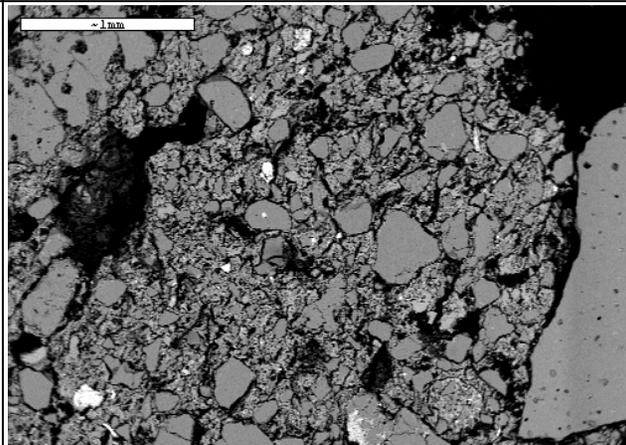
SEM-BS image of sample 204.3.201 showing the low fired section, with pronounced porosity.
