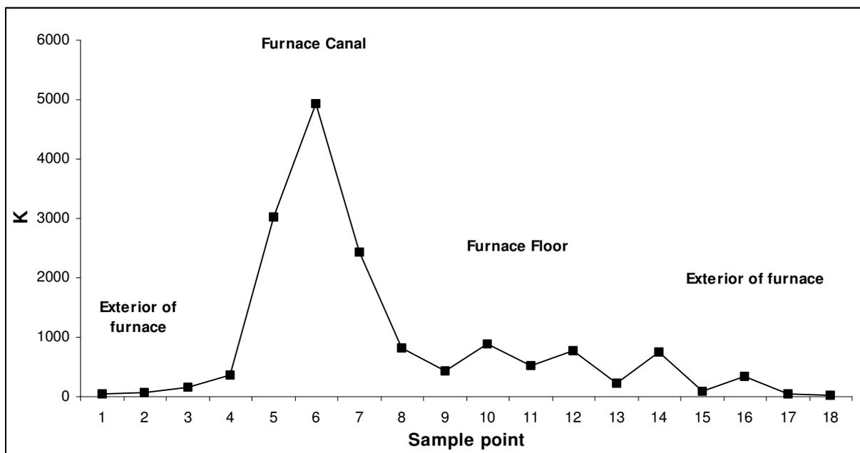
**Figure 5.** Context 121. Magnetic susceptibility ( $K$ ) measurements across the furnace from W-E.
