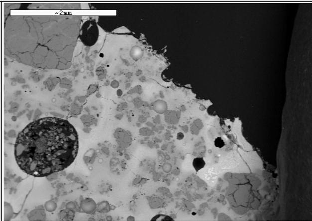
SEM-BS image of a detail within the vitrified area; it consists of partially melted and unaltered grains of quartz within a glassy matrix.
