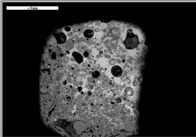
SEM-BS image of sample 204.3.201B showing two sections : a vitrified one(top right) and a low temperature heated one (bottom left) with a gradient of heating in between. This is a ceramic material
