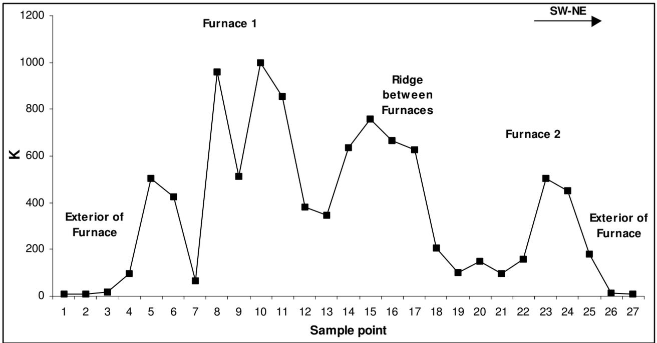
**Figure 3.** Context 5. Magnetic susceptibility measurements ( $K$ ) across the double furnaces from SW-NE.
