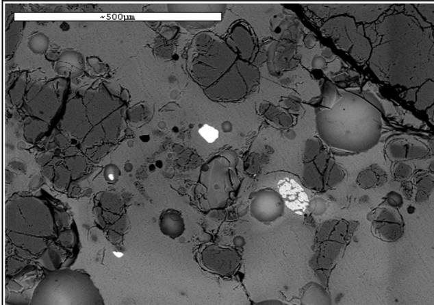
SEM-BS image of the vitrified section within sample 204.3.201B showing the presence of small inclusions of zircon and titanium iron oxides typical in clays.
