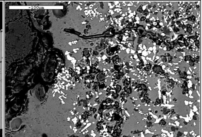
SEM-BS image of the low fired area within sample 204.3.201B showing the formation of iron oxides as a result of localised reducing conditions.
