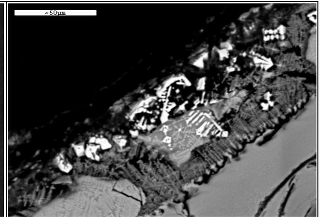
SEM-BS image of a detail within the surface of the vitrified area within sample 204.3.201B, showing the formation of iron oxides.
