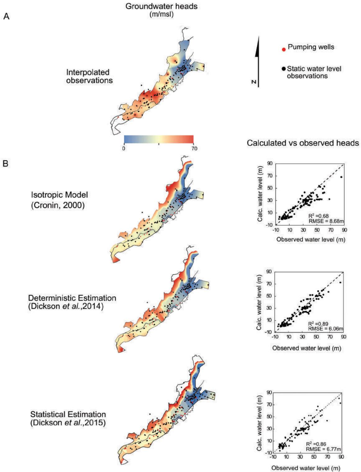
Figure 28.4. Maps of (A) interpolated static water levels observed in boreholes within the aquifer and (B) simulated groundwater heads (masl) for the isotropic, deterministic and statistical analyses. Model regressions show the fit of the models and the root-mean-square error values.
