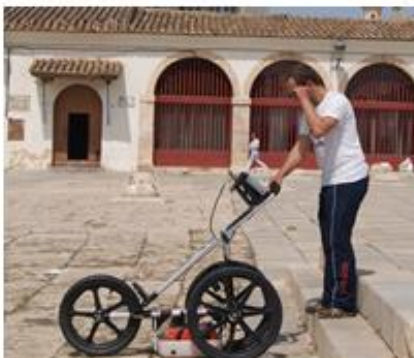
Figure 1.4. GPR (left) and thermography (right) (Ana Valls and David Montalvá, 2016)
