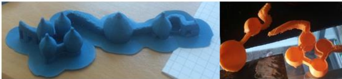
Figure 4.55. Wrong scale (left) and Wrong wall thickness (right)
