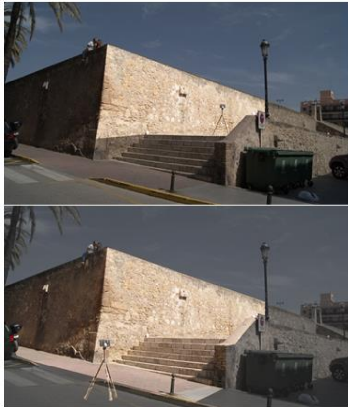
Figure 3.3 (Above) Bad scanner positioning, containing very inclined angles, (below) Good scanner positioning
