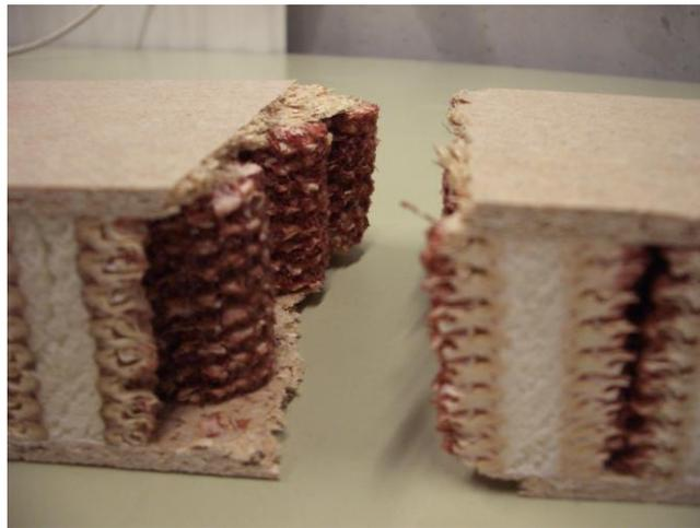
**Figure 29:** Sample collapsed after the test four points bending with surface layer of FPY and core layer of food-maize.
