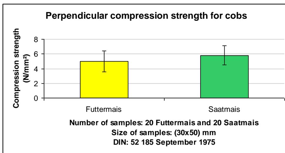
**Figure 35:** Perpendicular compression strength for samples of growing-maize (Saatmais) cobs and food-maize cobs (Futtermais). Units: (N/mm<sup>2</sup>). Number of samples: 20 of Futtermais and 20 of Saatmais. Size of samples: (30x50) mm. Following the standard DIN: 52 185 September 1975.
