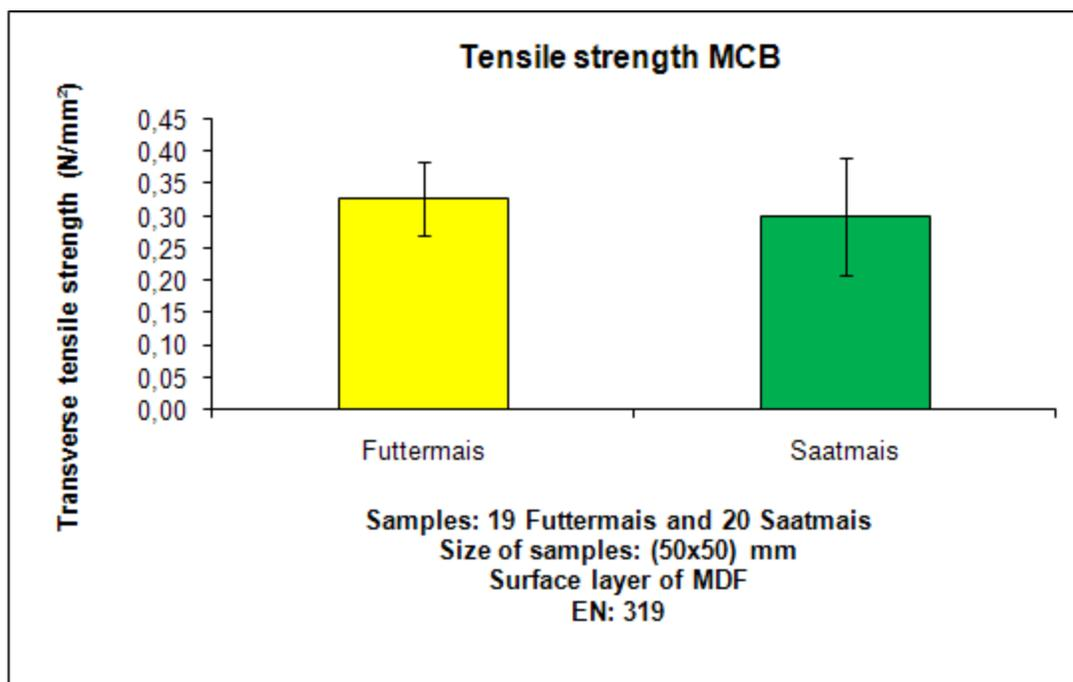
**Figure 32:** Tensile strength (N/mm<sup>2</sup>) from samples of core layer made with Futtermais and surface layer of MDF, and samples made with core layer of Saatmais and surface layer made of MDF. Size of samples is (50x50x40) mm. Number of samples: 19 samples with core layer of Futtermais and surface layer of 6 mm MDF, and 20 samples with core layer of Saatmais a surface layer of 6 mm MDF. Following the standard ÖNORM EN 319
