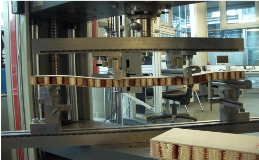
**Figure 28:** Determination of the bending strength by four points bending until the sampled is collapsed.
