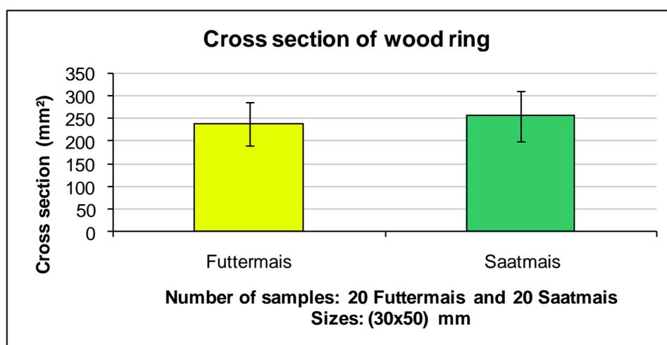
**Figure 30:** Cross section of wood ring (mm<sup>2</sup>) from samples of Futtermais and Saatmais. Size of each sample: (30x50) mm. Number of samples: 20 of Futtermais and 20 of Saatmais
