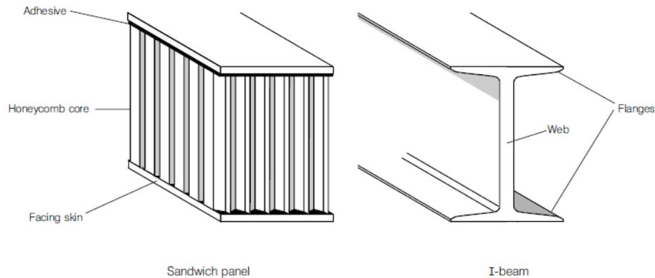
**Figure 9:** Shows the construction of a sandwich panel compared to I-beam (Hexcel Composites 2000)
