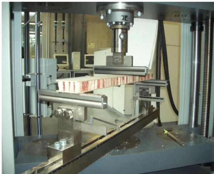
**Figure 27:** Determination for the modulus of elasticity by three-point bending with variable span. Size of sample (860 x100mm x thickness) mm. Surface layer of this sample made with MDF and with core layer of food-maize
