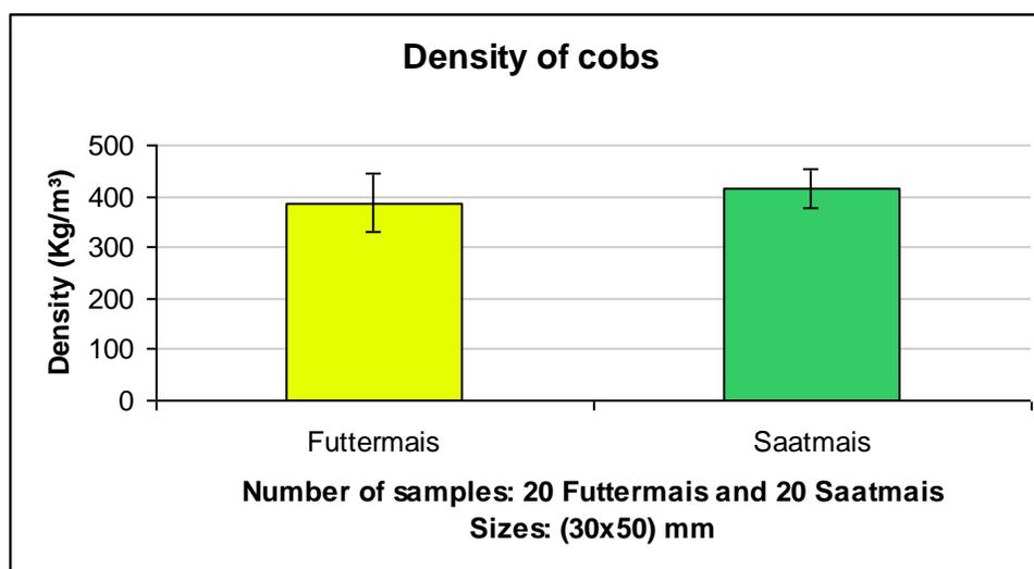
**Figure 31:** Density of cobs ( $\text{Kg/m}^3$ ) from samples of Futtermais and Saatmais. Size of each sample: (30x50) mm. Number of samples: 20 of Futtermais and 20 of Saatmais
