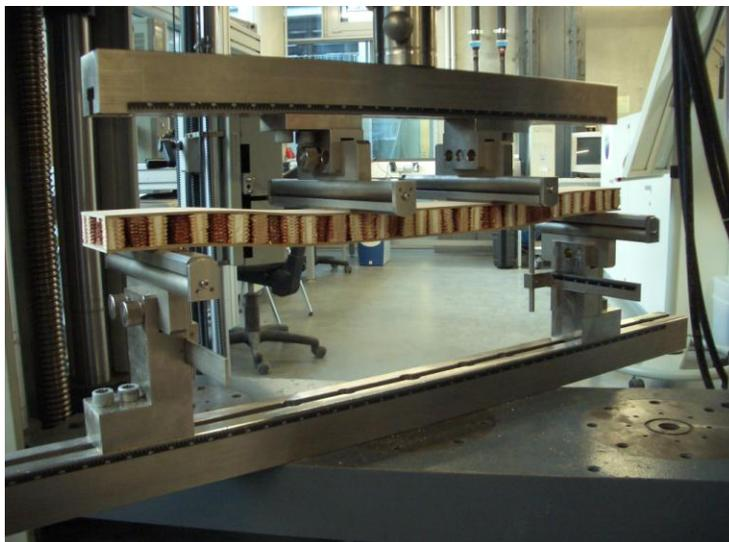
**Figure 24:** Samples of MCB during the bending test (4 Ptk).
