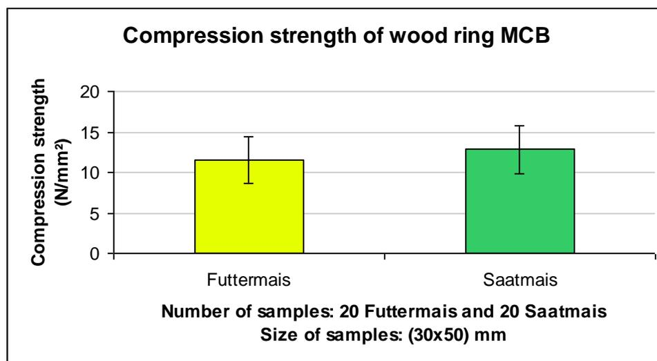
**Figure 36:** Perpendicular compression strength of wood ring, comparing samples of growing-maize (Saatmais) cobs and food-maize cobs (Futtermais). Units: N/mm<sup>2</sup>. Number of samples: 20 of Futtermais and 20 of Saatmais. Size of samples: (30x50) mm.
