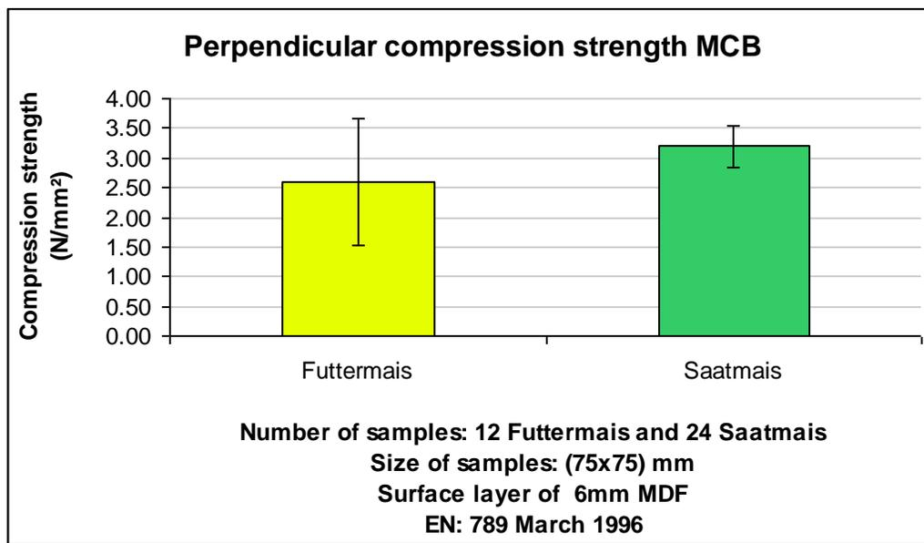
Figure 33: Perpendicular compression strength (N/mm<sup>2</sup>) from samples of core layer made with Futtermais and surface layer of 6mm MDF, and samples made with core layer of Saatmais and surface layer made of MDF. Size of samples is (75x75x40) mm. Number of samples: 12 samples with core layer of Futtermais and surface layer of MDF, and 24 samples with core layer of Saatmais a surface layer of MDF. Following the standard ÖNORM EN 789 March 1996
