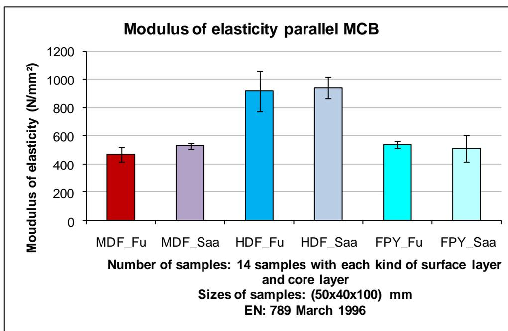
**Figure 41:** Modulus of elasticity parallel of MCB samples ( $N/mm^2$ ). Number of samples: 14 with each kind of surface layer and core layer. Samples of a surface layer of MDF
