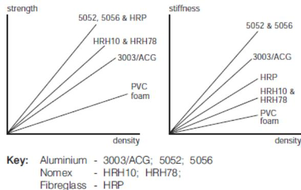
**Figure 10:** Comparison of different core materials between strength, stiffness and density (Hexcel Composites 2000)
