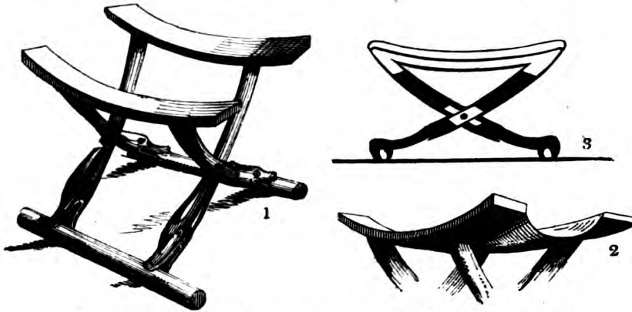
Fig. 1. A stool in Mr. Salt's collection, on the principle of our camp stools. 2. Shows the manner in which the leather seat was fastened. 3. A similar one from the sculptures, with its cushion.
