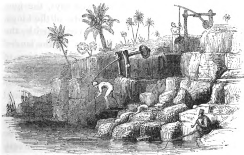
VIGNETTE D. Modern shadóf, or pole and bucket, used for raising water, in Upper and Lower Egypt.
