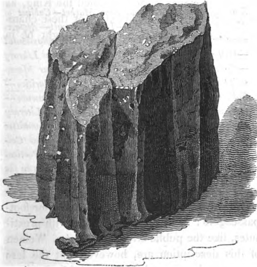
IGNEOUS BASALT , from the bottom of a Copper Furnace in Siberia. The original Specimen in the possession of the King of Sweden.
