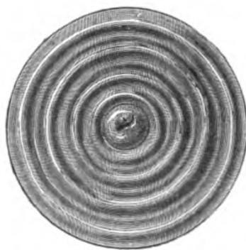
The bottom of the Cup, showing the terminal corrugations, as seen from below, and the central knob.
