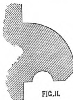
Fig. 2. String-course, South side of the Chapel.
