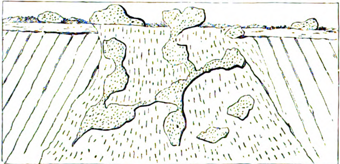
STRUCTURAL FORMATION OF GOLD-BEARING ROCKS, OPHIR, N.S.W.
