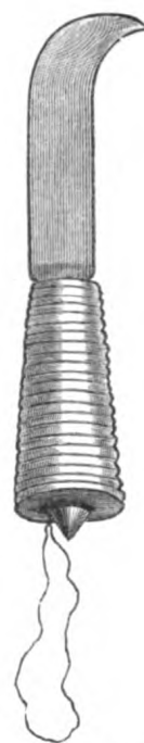
FIG. 84.—PERUVIAN KNIFE. METAL BLADE, SECURED IN A SLIT IN THE HAFT BY STRONG COTTON TWINE.
