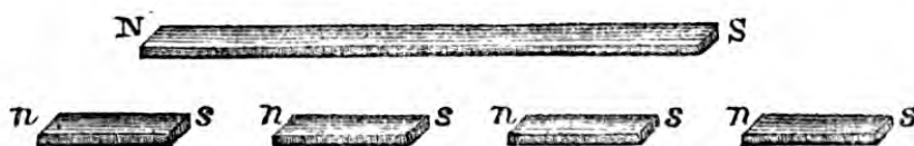
Fig. 9.—N, S, North and south poles of entire magnet. n, s , North and south poles of smaller magnets, into which the entire magnet is supposed to be broken.
