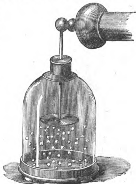
Fig. 106.—ELECTRICAL HAIL. Showing pith balls dancing between two metallic plates, one in connection with electrical machine at work, the other in connection with the earth.
