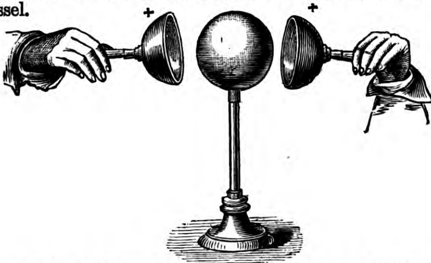
Fig. 81.—BIOT'S EXPERIMENT, showing tendency of electricity in insulated ball to escape to outer surface of insulated hemispherical caps.
