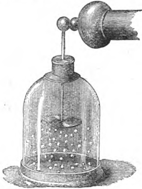
Fig. 98.—ELECTRICAL HAIL. Showing pith balls dancing between two metallic plates, one in connection with electrical machine at work, the other in connection with the earth.
