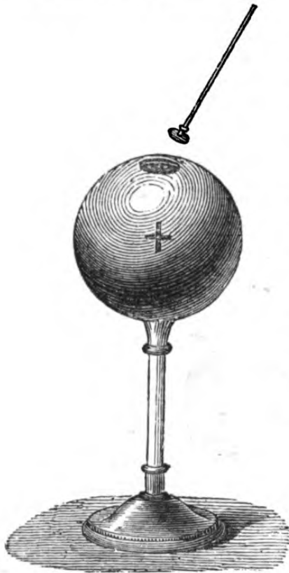
Fig. 82.—Showing mode of testing interior of HOLLOW ELECTRIFIED BALL , by means of PROOF-PLANE .
