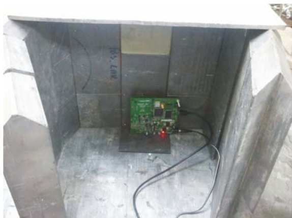
Figure 7. Photograph of the board placed inside the shield
