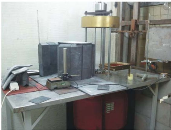
Figure 3. The lead collimation system
