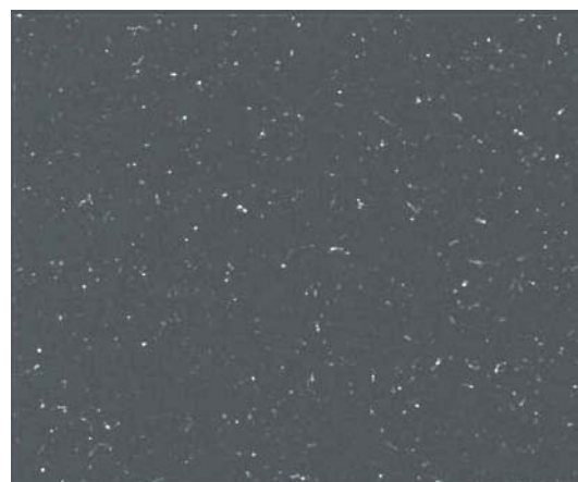
Figure 8 . Acquired image from the CMOS camera, in dark conditions, during irradiation. Primary (single white pixels) and secondary electrons interactions (tracks) are clearly evidenced at short exposure times
